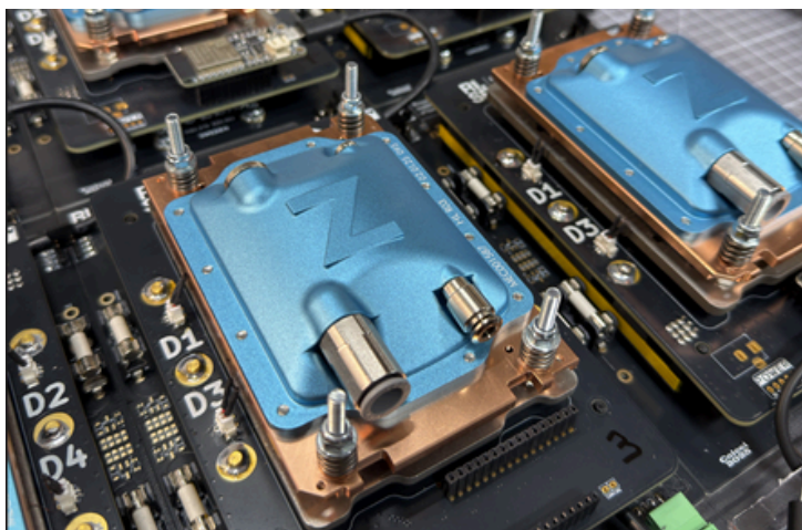
ZutaCore's liquid cooling technology
