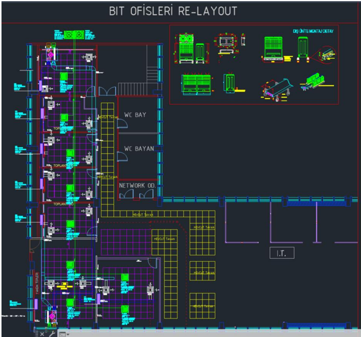
Figure 2.117: New part of the IT office (with the floor-standing fan coil system, in bright purple, and AC system, in green).
