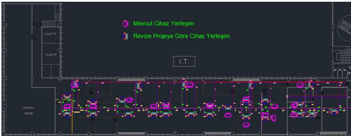
Figure 2.116: Old part of the IT office (with the ceiling-mounted fan coil system).
