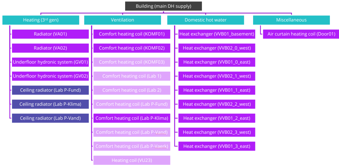
Figure 2.4: AAU pilot system overview (Dark purple indicates that the supply temperature used is after the mixing loop or there is no mixing loop. Light purple indicates that the supply temperature is measured before the mixing loop, thus not being the temperature directly used by the system. Those in dark blue are missing energy use measurements, thus not allowing them to be analyzed directly).
