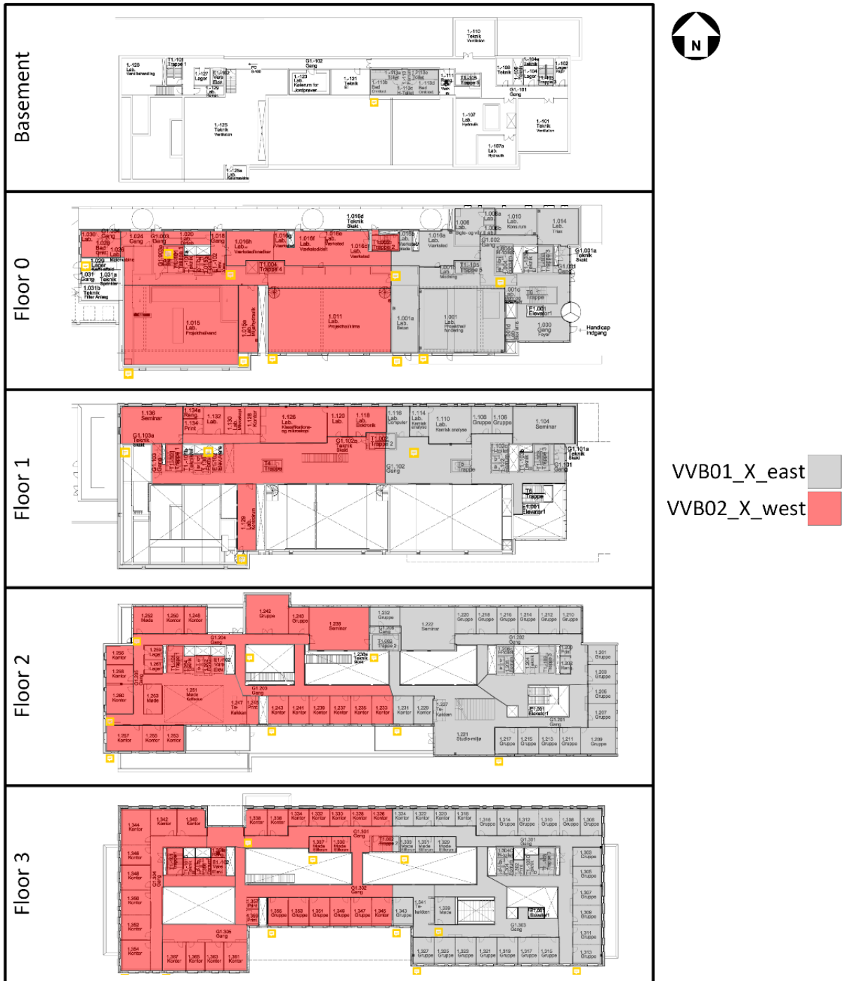
Figure 2.11: Areas covered by the different domestic hot water systems in the AAU pilot. The X denotes the floor, going between 0 and 3 for both, while the VVB01 also has the basement.
